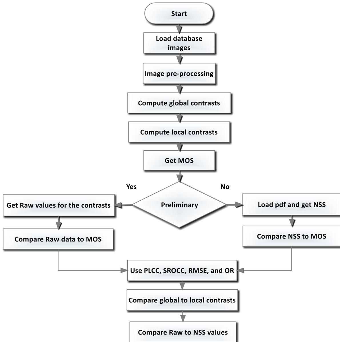
Fig. 4. Experiments block diagram.
